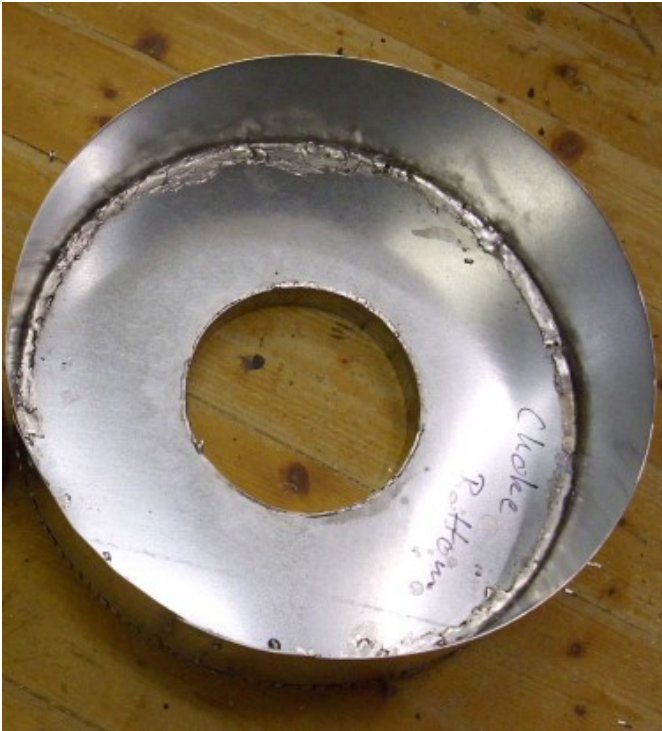
Figure 14: Choke ring soldered
