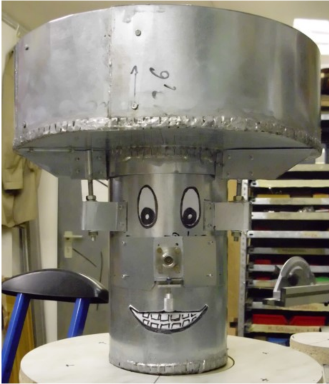
Figure 15: Final feed horn
