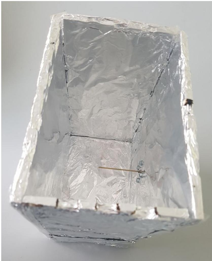
Figure 22: Wooden box waveguide
