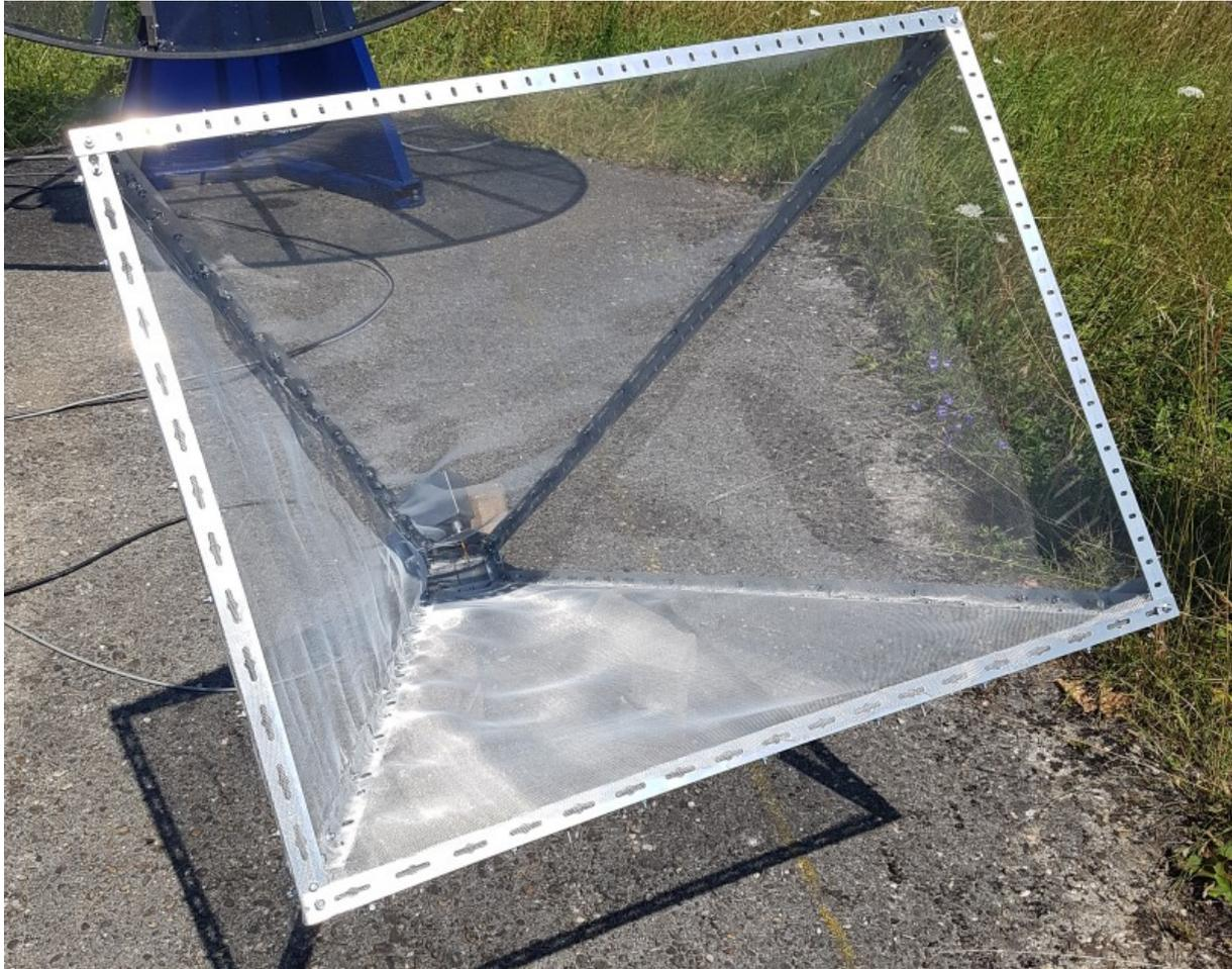
**Figure 35: Horn of Plenty Antenna**
