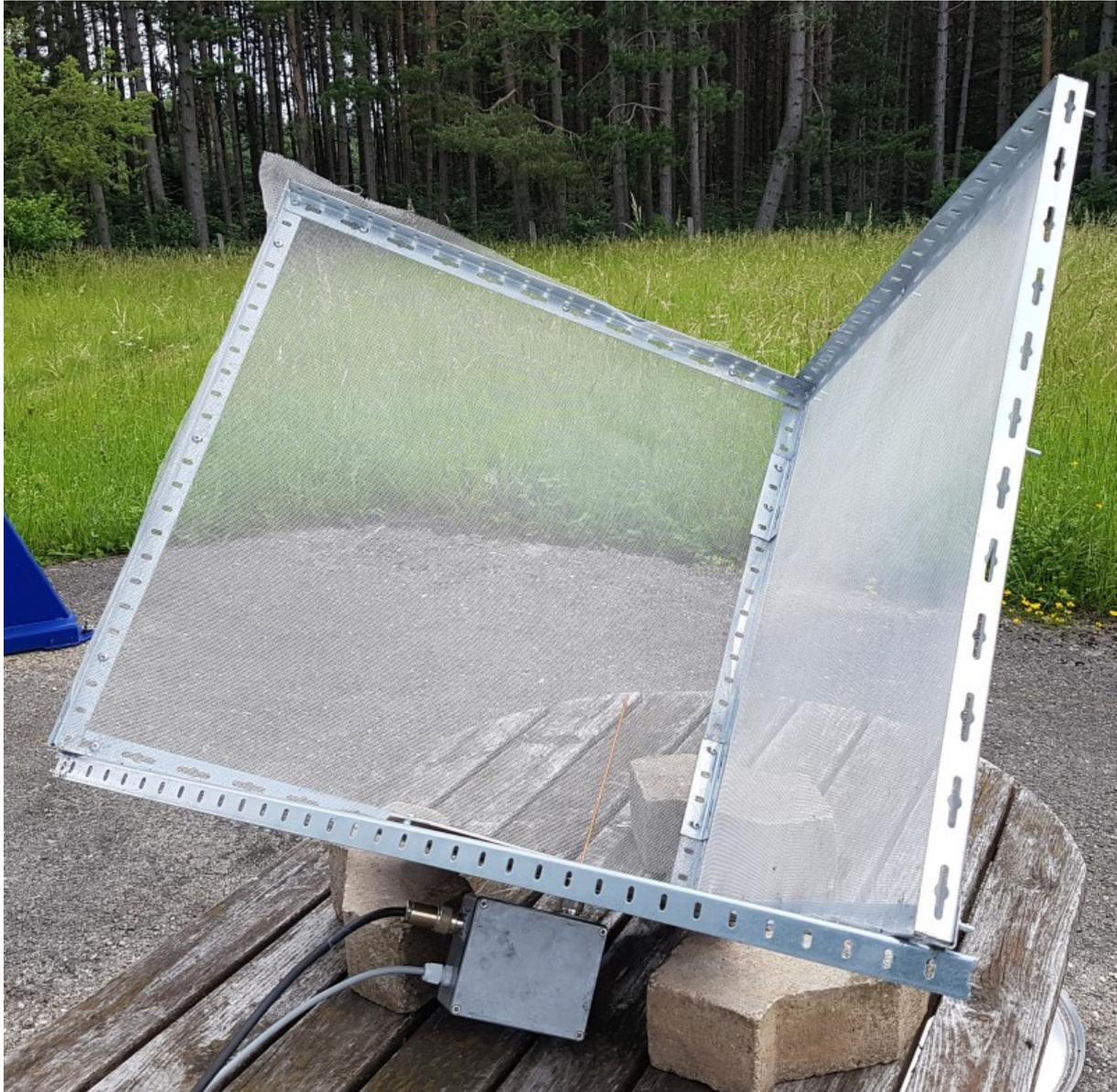
Figure 33: 3D corner antenna
