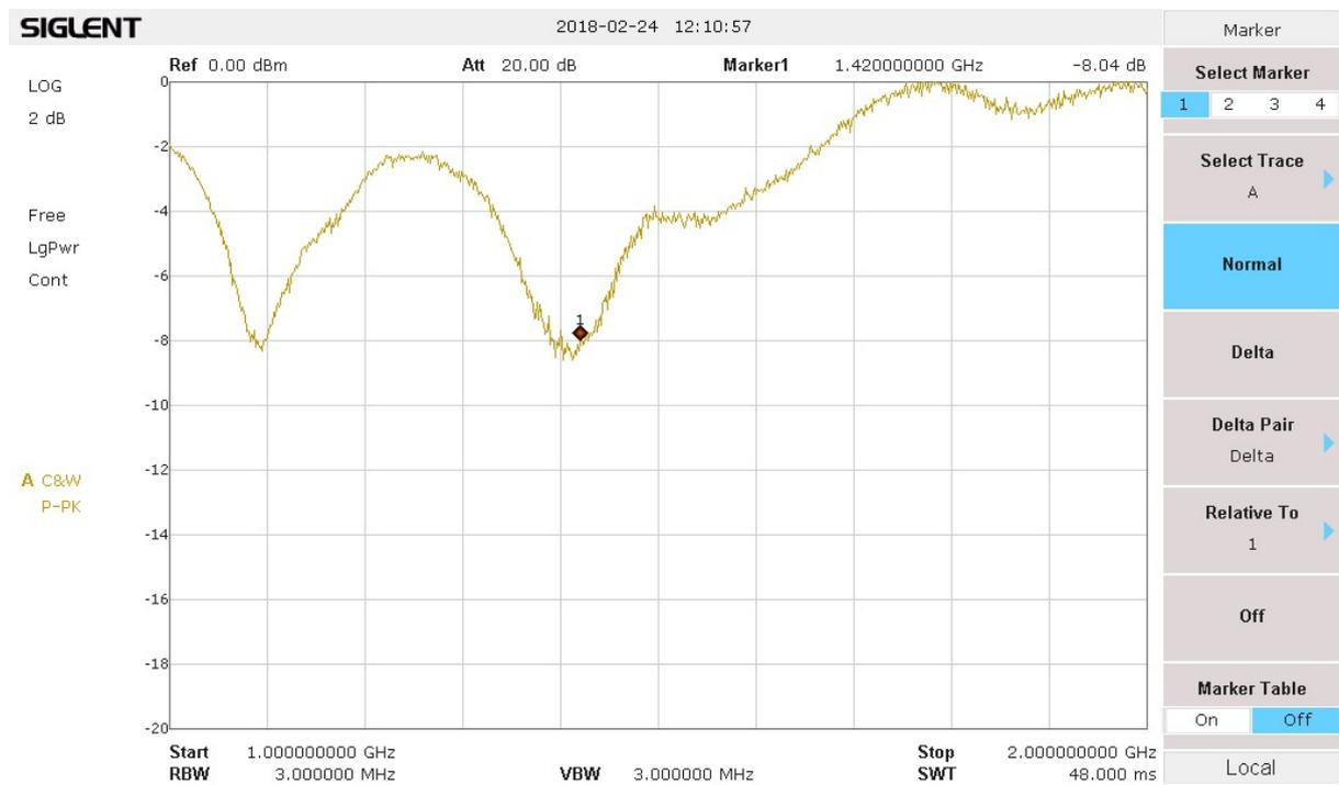
**Figure 16: Dipole with reflector (variant) return loss measurement**
