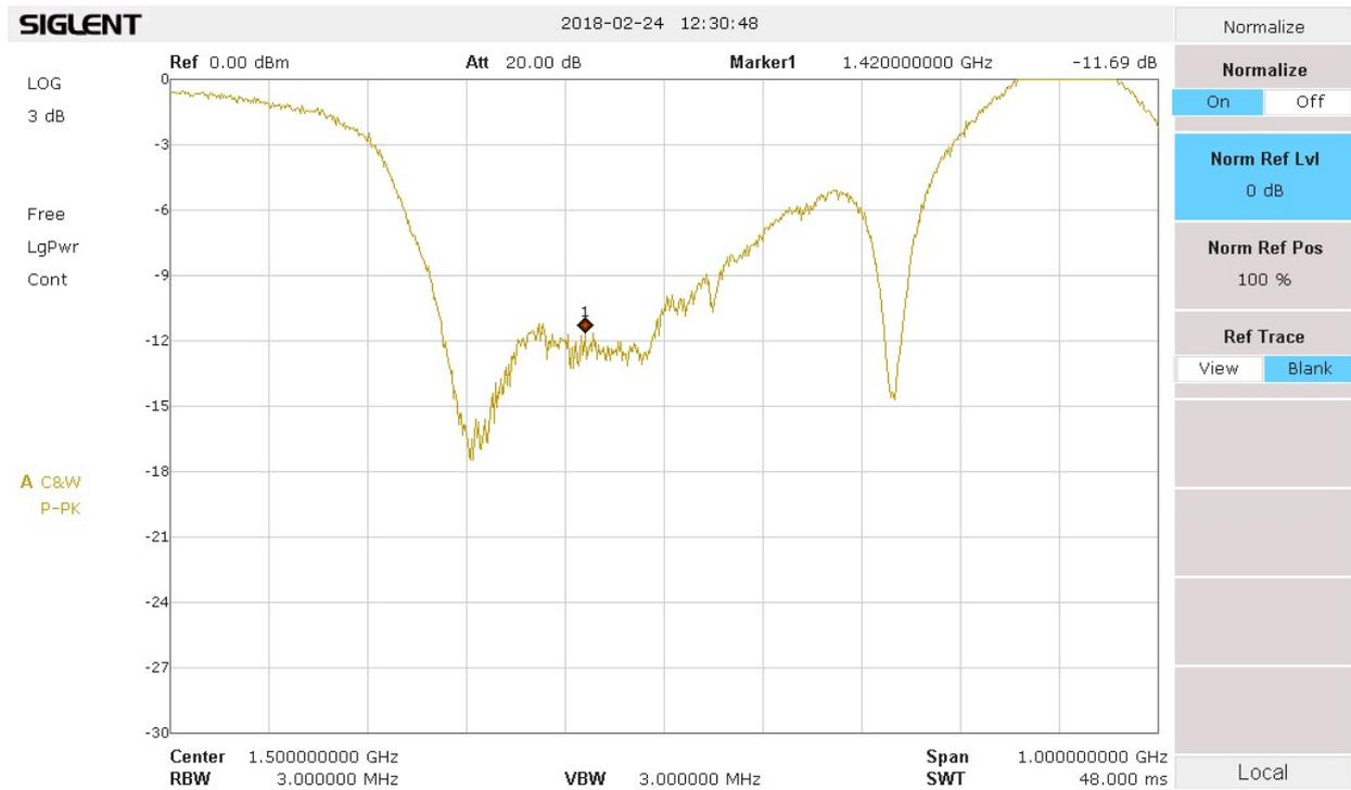
**Figure 19: Circular Waveguide Return Loss**
