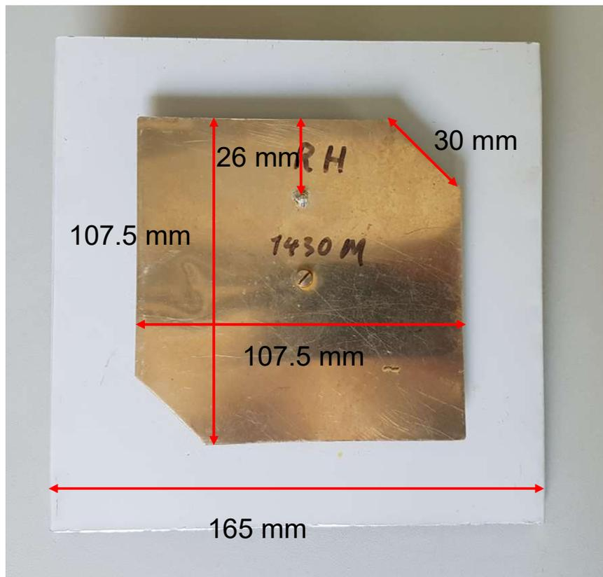
**Figure 24: Air gap patch antenna top view**
