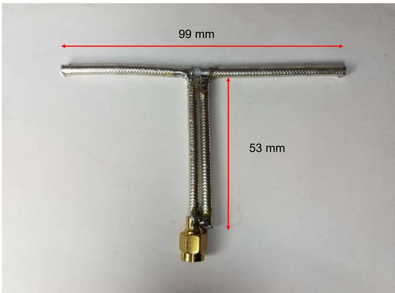
Figure 9: Dipole antenna
