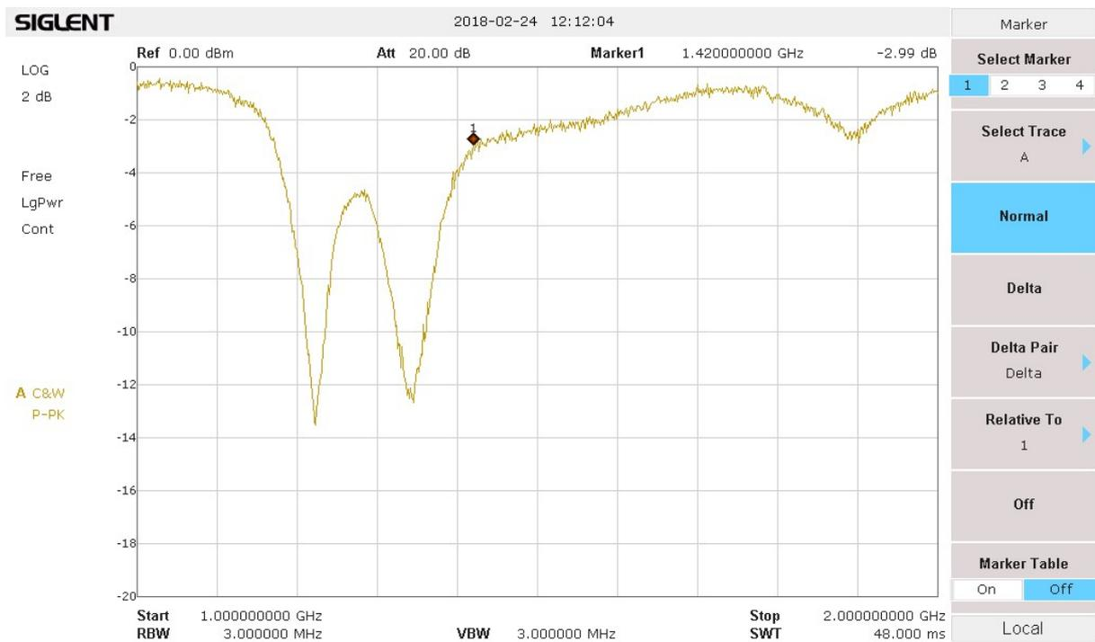
Figure 26: Air gap patch antenna return loss
