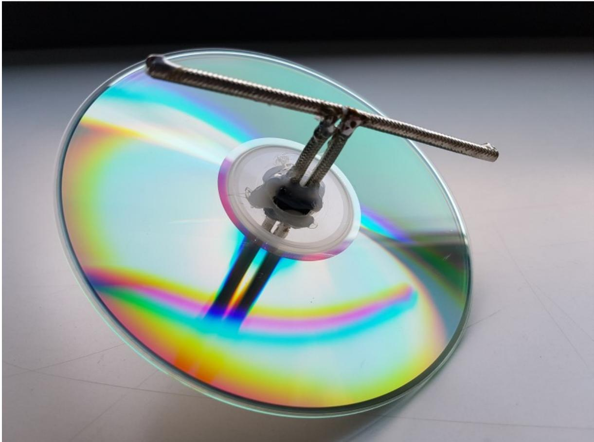
**Figure 12: Dipole with CD as reflector**
