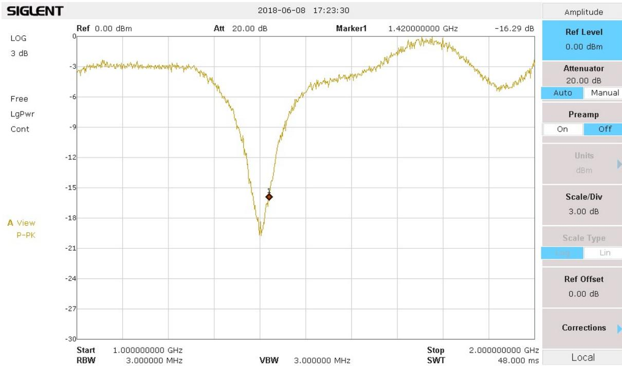
Figure 34: 3D corner antenna return loss measurement
