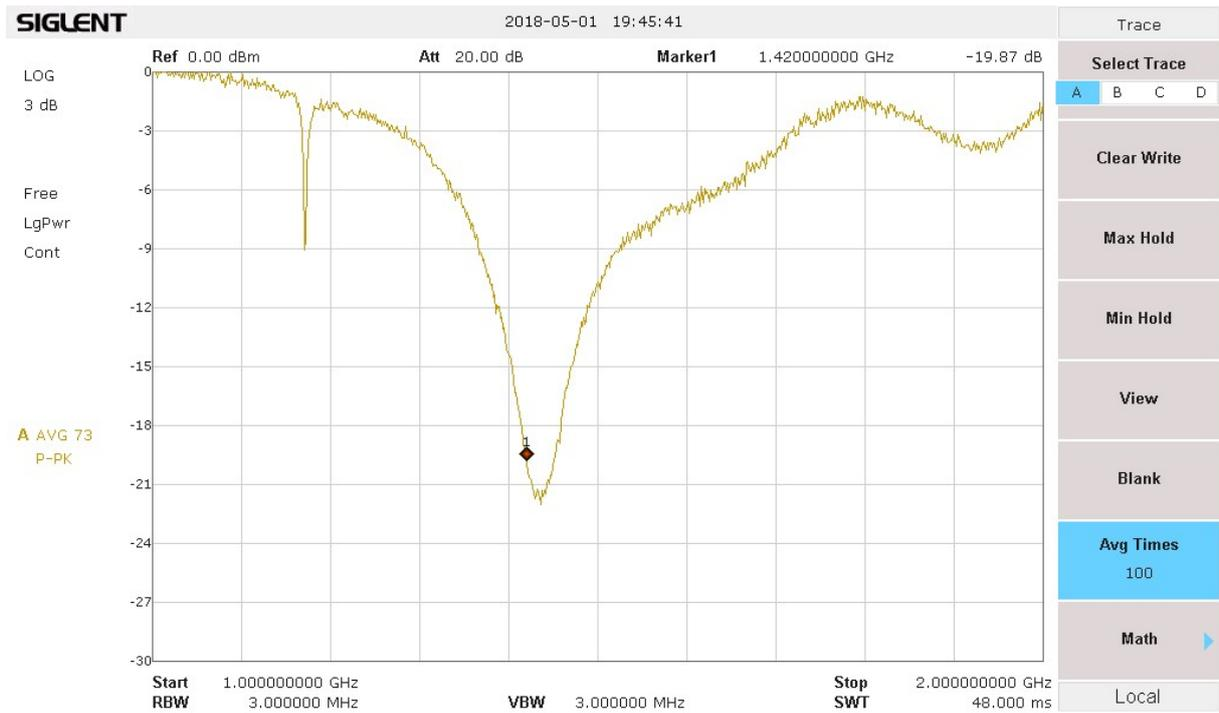
**Figure 13: Dipole with reflector return loss measurement**
