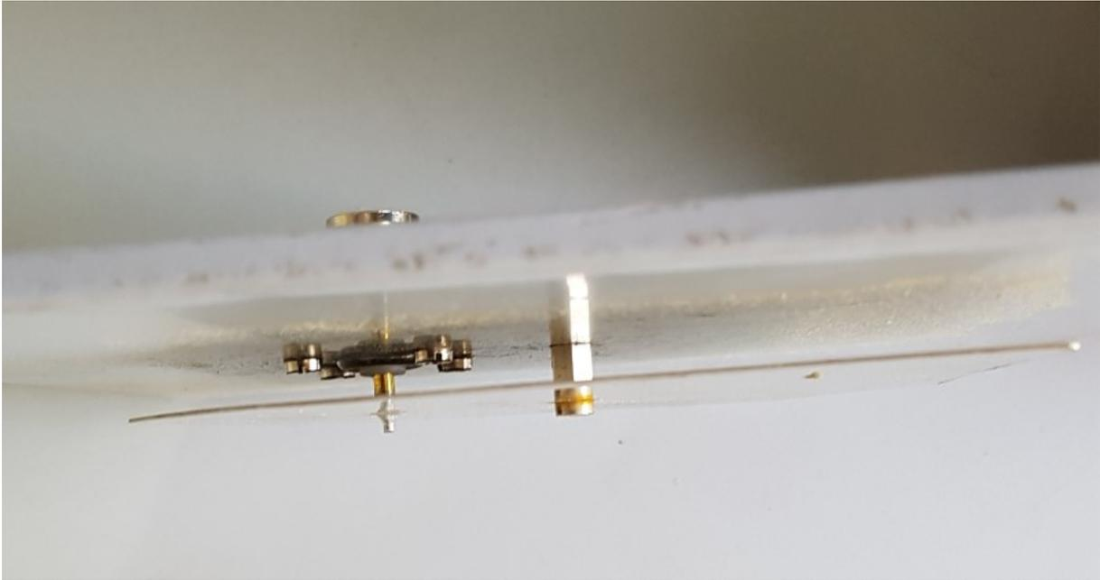
Figure 25: Air gap patch antenna side view
