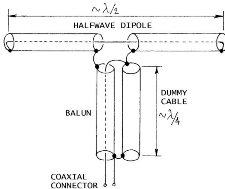
**Figure 10: Dipole antenna electrical connections**
