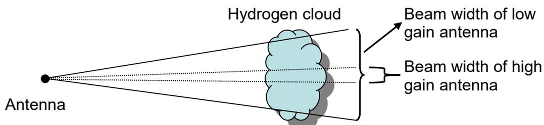
Figure 40: Geometry of antennas with different gain
