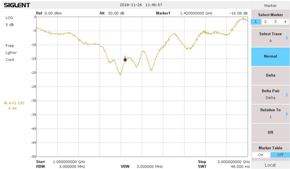
**Figure 36: Return loss of horn of plenty antenna**
